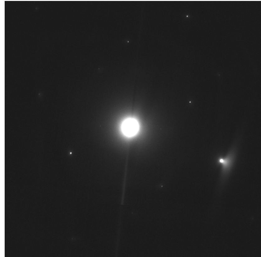
Si near a 2-beam condition
